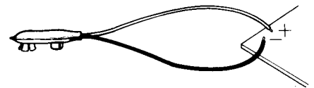
Figure 5a: Basic 'battery snap' wiring without switch. The black lead in all cases is negative.
